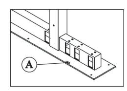
4. Slide cross beam over both tabs on leg.
