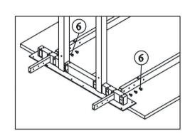
9. Inserts spacers (part 4) under the cross beam. Use wood screws (part 5) to attach the beam to table top.
