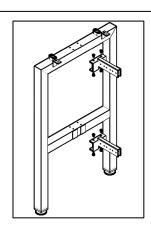
3. Slide cross beams over CBB ends and attach with M6 x 12 mm bolts.
