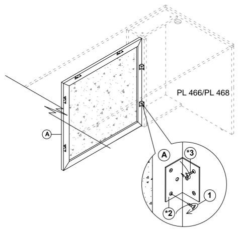
Attach L-Bracket #2 to Glass Modesty Panel (A) with hole marking (6 pcs in total) and to PL 466/PL468 by using 12pcs x screw #1 & 18pcs x screw #3 as shown.
