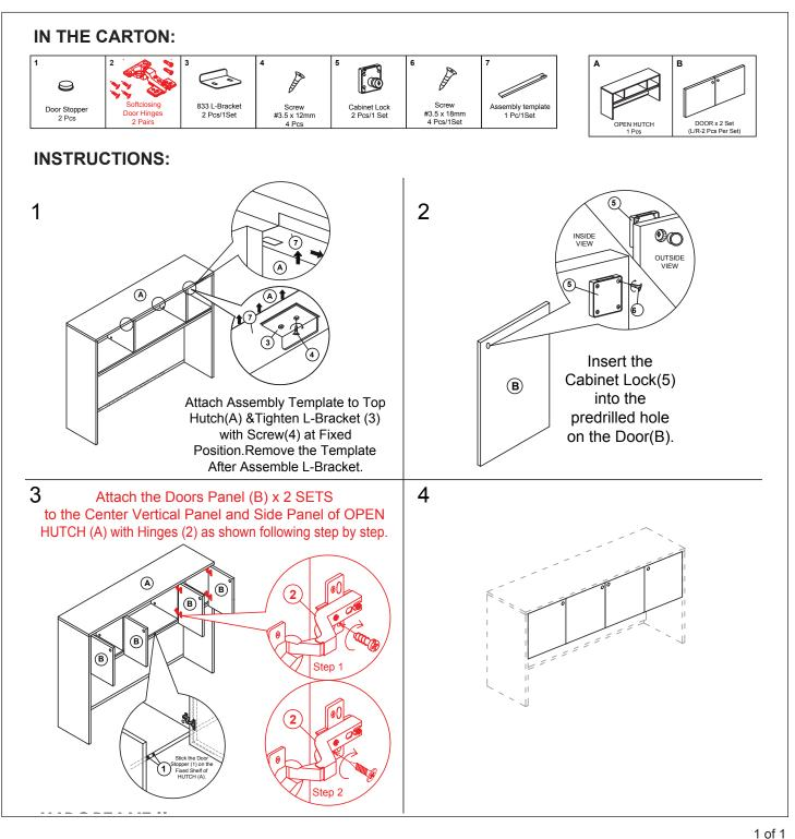
Do not tighten any screws or bolts until the unit is completely assembled.
