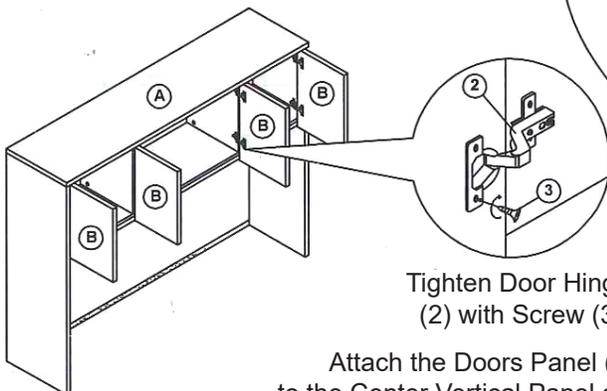
Tighten Door Hinges (2) with Screw (3).
