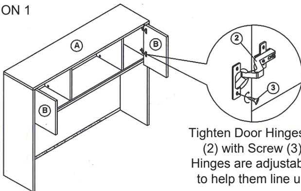
Tighten Door Hinges (2) with Screw (3). Hinges are adjustable, to help them line up.
