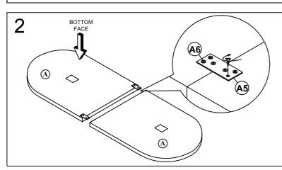
Attach the Flat-Bracket (A2) to two Top Panel (A) as shown. Tighten Screws (A3) securely.
