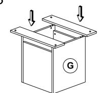
Attach Cube Base Support (G) by using Cam Lock (G1) and Klix Cam (G2).
