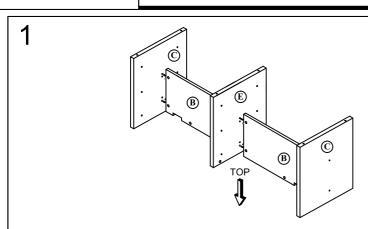
Attach the two End Base (C) and Center Base (E) to Modesty Panel (B) by using Cam Lock (C1) and Klix Cam (C2).
