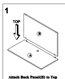
Panel(A) by using Cam Lock(1) and Klix Cam(2).
