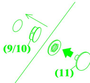
**Insert the Hole Plug (9/10) and D-nut Cap (11) to all drill hole of the other edge of Side Panel (C) and Back Panel (B) which the hole are not in use.**
