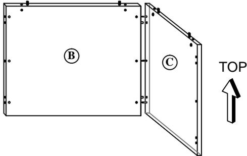
**Attach Back Panel(B) to Side Panel(C) by using Wood Dowel(12), Cam Lock(1) and Klix Cam(2).**
