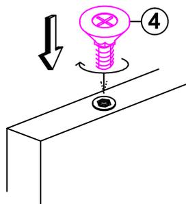
**Screw Adjustable Glide(4) into bottom of Back Panel(B) and Side Panel (C).**
