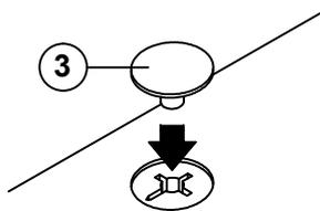
**Attach Housing Cap (3) to all Klix Cam(2) by pushing along thought center of cam.**
