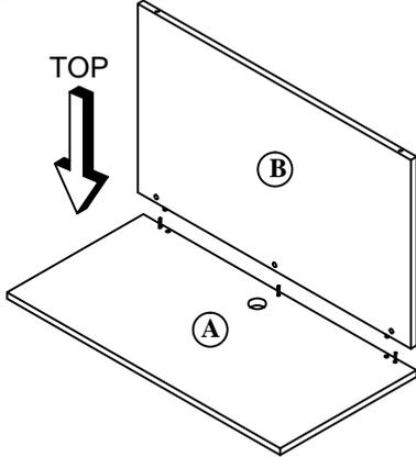
**Attach Back Panel(B) to Top Panel(A) by using Cam Lock(1) and Klix Cam(2) as shown in Detail- X.**
