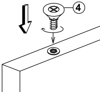
**Screw Adjustable Glide(4) into bottom of Side Panel.**
