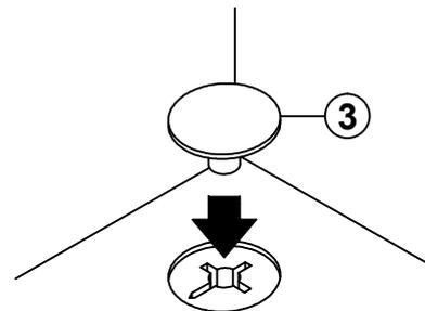
**Attach Housing Cap(3) to all Klix Cams(2) by pushing neck through center of cam.**
