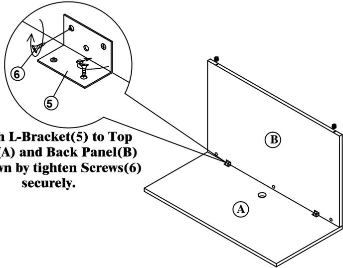
**Attach L-Bracket(5) to Top Panel(A) and Back Panel(B) as shown by tighten Screws(6) securely.**
