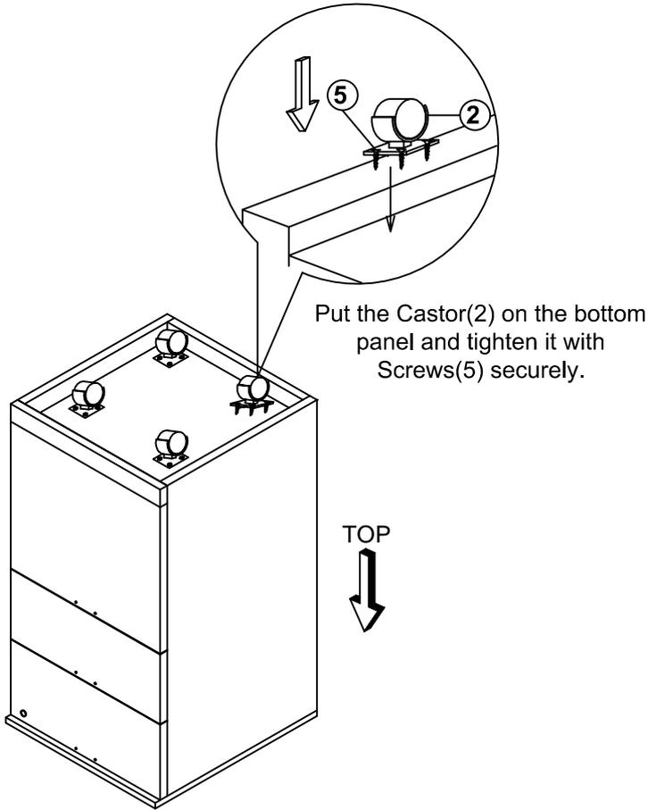
Put the Castor(2) on the bottom panel and tighten it with Screws(5) securely.
