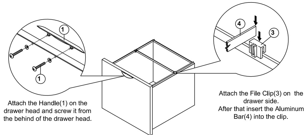
Attach the Handle(1) on the drawer head and screw it from the behind of the drawer head.
