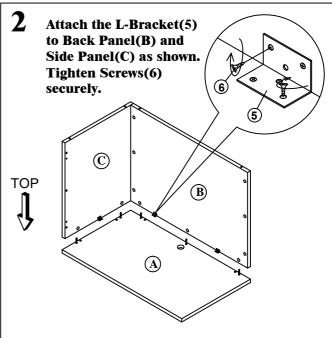
Attach the Back Panel(B) and Side Panel(C)
