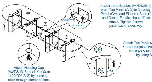
from Top Panel (A/D) to Modesty Panel (G/H) and Eleptical Base (I) and Center Eleptical base (J) as shown. Tighten Screws (A6/D6/J7/I8) securely.
