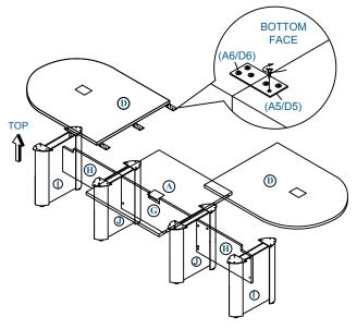
Attach the Flat-Bracket (A5/D5) to two Top Panel (D) and Top Panel (A) as shown. Tighten Screws (A6/D6) securely.
