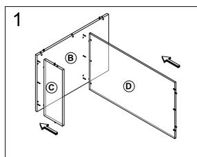
Attach the Center Panel (D) and End Panel (C) to Side Panel (B) by using Cam Lock (1) and Klix Cam (3).
