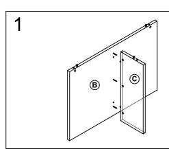
Attach the Side Center Panel (C) to Side Panel (B) by using Cam Lock (1) and Klix Cam (2).
