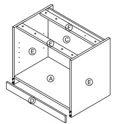
Attach the Front Rail (D) to Both Side Panel (E) by wood dowel.
