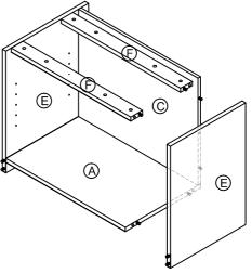
Attach the another Side Panel (E) to Hanging Panel (F) and Back Panel (C) and Bottom Panel (A) by using Cam Lock (1) and Klix Cam (2).
