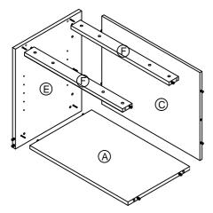
Attach the Bottom Panel (A) and Hanging Panel (F) and Back Panel (C) to Side Panel (E) by using Cam Lock (1) and Klix Cam (2).
