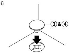
Attach Housing Cap (3/4) to all Klix Cams (2) by pushing neck thought center of cam.
